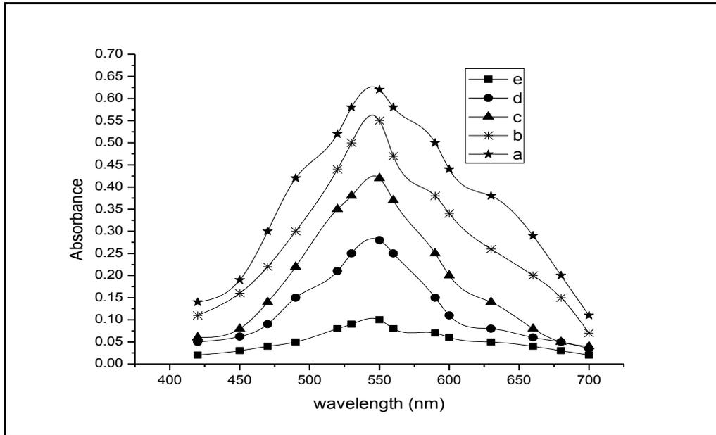
**Fig. 3.** Absorption spectra of  $\text{KMnO}_4$  ( $60 \mu\text{g mL}^{-1}$ ) after treating with: a. 0, b. 5, c. 10, d. 20 & e. 30  $\mu\text{g mL}^{-1}$  DEC.
