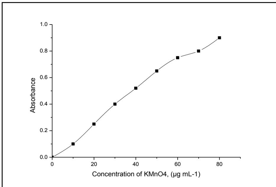
**Fig. 4:** Linear relation between absorbance at 550 nm and  $\text{KMnO}_4$  concentration in  $\text{H}_2\text{SO}_4$ .
